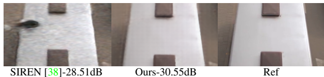
Figure 9: SIREN struggles with high-frequencies in temporal domain. Our model faithfully reconstructs high-frequencies in both the spatial and temporal dimensions. We show the last frame of a video segment before a jump-cut to a different shot. This is a sharp transition in time, which SIREN struggles to model accurately.
