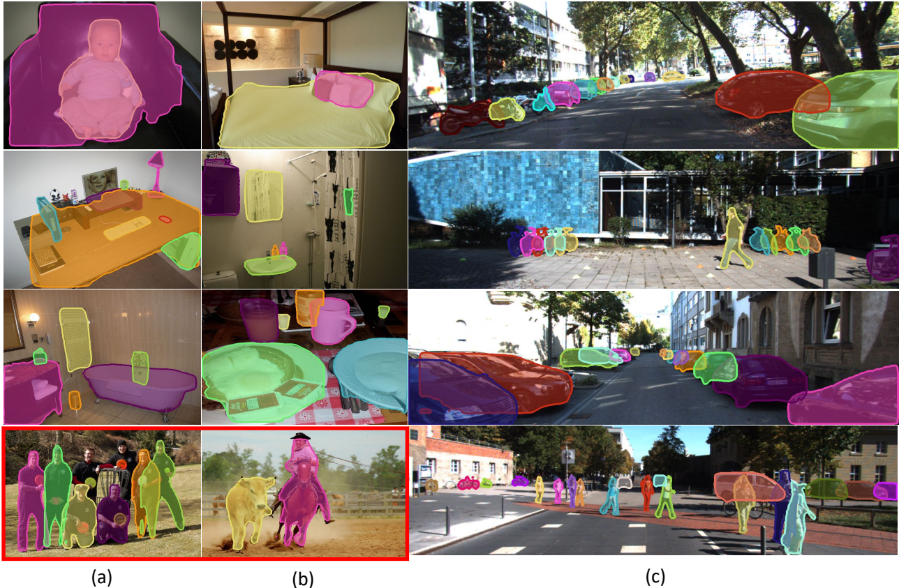
Figure 7. Qualitative results for amodal instance segmentation on COCOA-test are shown in (a) and (b), and on KINS-test in (c). All of them are successful cases except the failure cases are marked red. The first failure case is about incomplete person detections and the second failure case is about merging masks of a person and horse.
