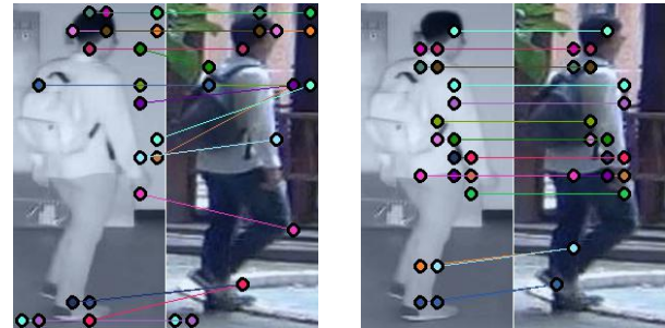
Figure 1: An example of dense cross-modal correspondences between RGB and IR images from the SYSU-MM01 dataset [36]. For the visualization purpose only, we show the top 20 matches according to similarities between local person representations learned without (left) and with (right) our approach. Our person representations are robust to the cross-modal discrepancies, while being highly discriminative, especially for person regions. (Best viewed in color.)
