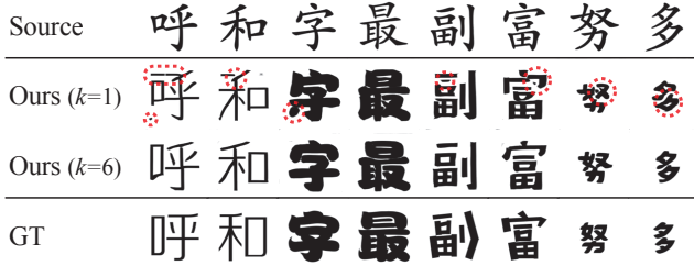
Figure 8. Generated samples of the models having different number of heads ( k ). The samples generated with four reference glyphs by the single-headed model and multi-headed model are shown. We highlight the defects in red dotted circles that appeared in the images generated by the single-expert model.
