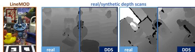
Figure 1: **Differentiable Depth Sensor Simulation (DDS) for the generation of highly-realistic depth scans.** DDS works off-the-shelf, but can be further optimized unsupervisedly against real data, yielding synthetic depth scans valuable to the training of recognition algorithms (demonstrated here on LineMOD dataset [21]).
