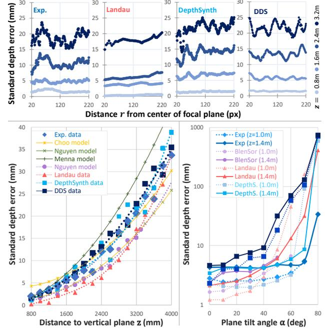
Figure 5: **Sensor noise study.** Given a flat surface placed at various distances  $z$  and tilt angles  $\alpha$  w.r.t. the sensor, we plot the standard depth error as a function of  $r$  distance to the focal center in screen space, of  $z$ , and of  $\alpha$ ; for actual and simulated *Kinect VI* scans and statistical sensor models.
