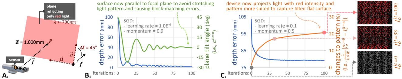
Figure 6: **Optimization of scene and sensor parameters** via simulation, to improve sensor precision in controlled use-cases. A. Experimental setup *c.f.* Section 4.1; B. Optimization of the scene parameters (*e.g.*, pose) to reduce sensor standard error; C. Optimization of the sensor (*e.g.* pattern structure and frequencies) to improve its accuracy w.r.t. such scenes/materials.
