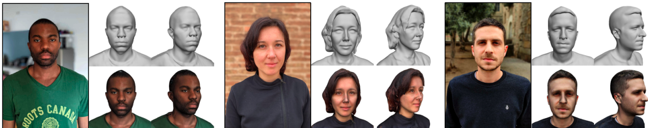
Figure 1. We introduce H3D-Net, a method for high-fidelity 3D head reconstruction in the wild. Our method estimates a signed distance function (SDF) of the head by optimizing a coordinate-based neural network on a small set of input images. This optimization process is constrained by a pre-trained probabilistic model of 3D head SDFs to obtain plausible shapes in few-shot setups. The figure shows the 3D head reconstruction of three scenes obtained with the proposed method from only three images with associated masks and camera poses.
