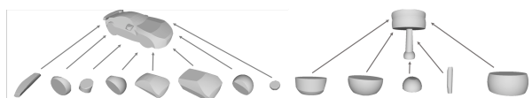
Figure 5. Two examples show how a car and a lamp can be constructed with a small number of parts of intersection nodes. The decomposition is compact, interpretable, and consistent with the semantic parts of cars and lamps. Note that we only show the visible parts.
