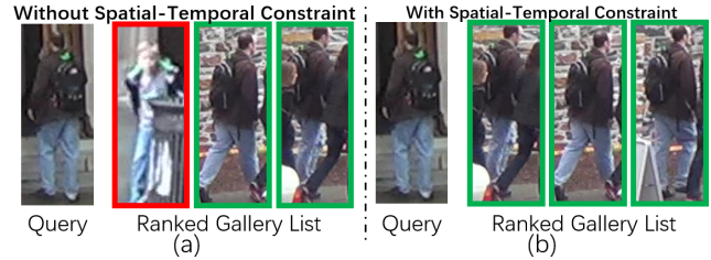
Figure 4. (a): The appearance of the pedestrian in the red bounding box, who is mistakenly ranked first, is similar to the query image. (b): The incorrect pedestrian is filtered out by the spatial-temporal constraint.
