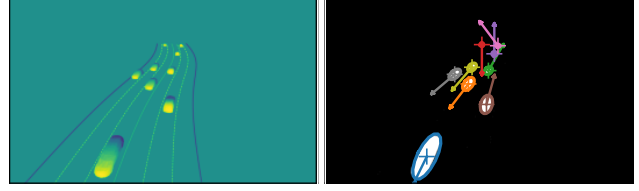
Figure 4. Visualisation of the representation r_b extracted for car mask b . Left : Synthetic scene. Right : ellipses (1 st and 2 nd order moments) and normalized motion (arrows) on top of binary car masks. More examples are in the supplementary.
