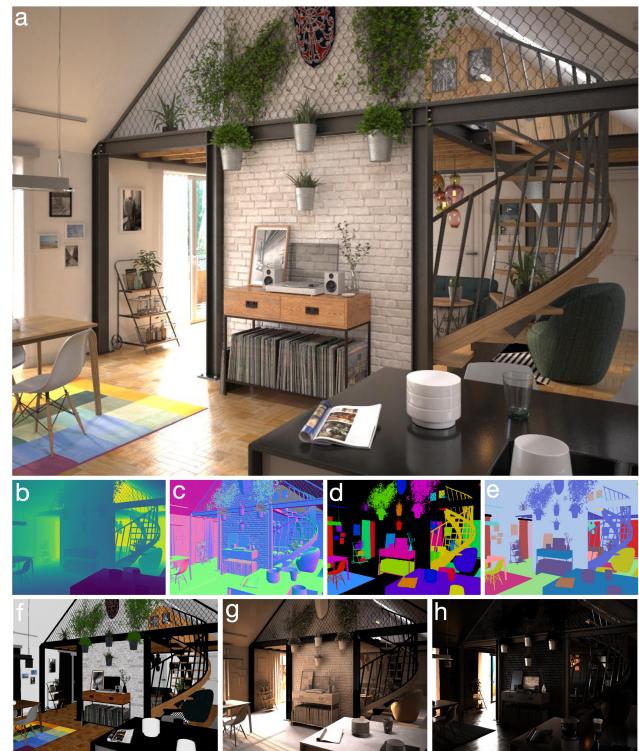
Figure 1. Overview of the Hypersim dataset. For each color image (a), Hypersim includes the following ground truth layers: depth (b); surface normals (c); instance-level semantic segmentations (d,e); diffuse reflectance (f); diffuse illumination (g); and a non-diffuse residual image that captures view-dependent lighting effects like glossy surfaces and specular highlights (h). Our diffuse reflectance, diffuse illumination, and non-diffuse residual layers are stored as HDR images, and can be composited together to exactly reconstruct the color image.
