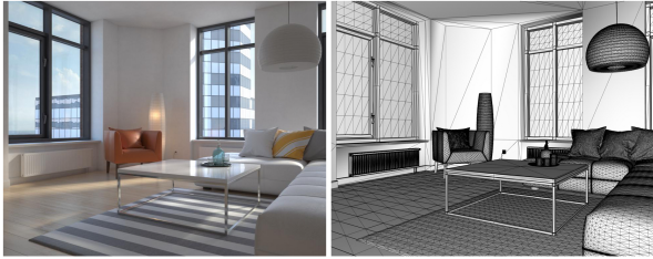
Figure 5. Color and wireframe renderings of a typical scene. In the wireframe rendering, we observe that the salient objects (e.g., chair, couch, lamp) are more finely tessellated than the non-salient objects (e.g., walls, floor, ceiling). This observation motivates our view sampling heuristic that takes triangle density into account, and does not require an input scene to be semantically labeled.
