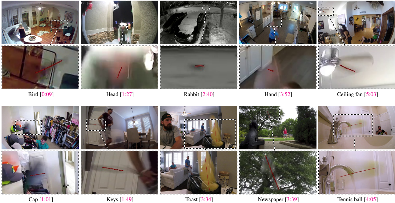
Figure 2. Examples of fast moving object (FMO) retrieval on YouTube videos by our method running in real-time. Top: frames from a 10-minute surveillance footage [youtu.be/CkVJyAKwByw]. Bottom: frames from a 5-minute trick-shot video [youtu.be/A2FsgKoGD04]. For each image, the detected FMO and its trajectory is shown as a red line in a close-up below. The object description contains a digitally clickable link to the timestamp when the event happened, in [minutes:seconds] format.
