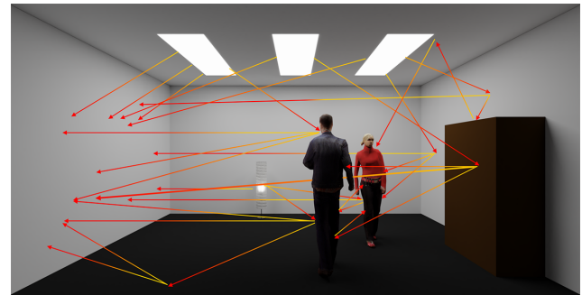
Figure 1: The light originating from the lamps takes infinitely many paths to reach the wall on the left. Motion of people in the room changes the mutual visibility between the wall and the rest of the scene, which induces subtle changes in patterns of light observed on the wall. Notice that there are no direct shadows, as the persons do not occlude the direct paths connecting the left wall and the lamps.
