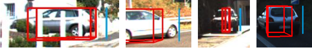
Figure 3. Comparisons between the predicted eight projected corners (red boxes) and predicted visual height (blue lines). Predicting the eight projected corners fails under challenging cases, such as occlusion, truncation, and extreme lighting conditions, while predicting the visual height is more simple and robust. The images are from the val subset of the KITTI validation split [6].
