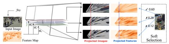
Figure 3. Illustration of the proposed SHOT. Each feature map will be projected with a stack of homographies and the projection results are selected softly to form a proper screen $\rightarrow$ BEV projection.
