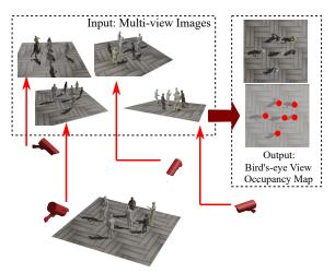
Figure 1. The task of multi-view pedestrian detection: Given a batch of synchronized images captured from different view angles, our goal is to predict an occupancy map of the scene.
