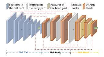
Figure 5: Overview structure of the FishNet. We insert our DEPLA module in the UR and DR blocks (rendered in red) where the feature aggregation happens.
