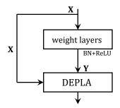
Figure 6: Integrate DEPLA into residual block
