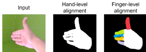
Figure 8. The alignment evaluation is conducted on two levels. For hand-level alignment, we evaluate only the silhouette of the whole hand between the prediction and ground truth. For finger-level alignment, we evaluate individual fingers and palm. Finger-level alignment is more demanding than hand-level alignment.
