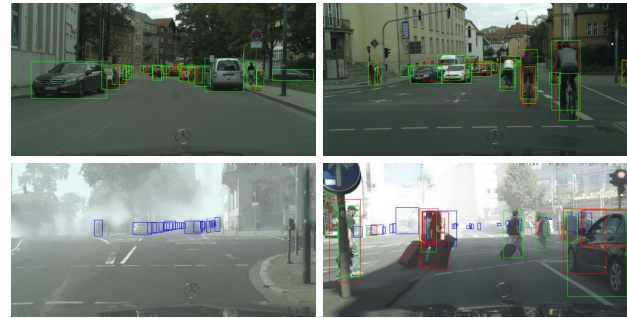
Figure 1. Detected objects in source domain (1st row) and target domain (2nd row). The results are collected from a detector only trained on Cityscapes. Green, red, and blue boxes are true positives, false positives and false negatives. We can observe that many targets have been missed in the domain-shifted Foggy Cityscapes.
