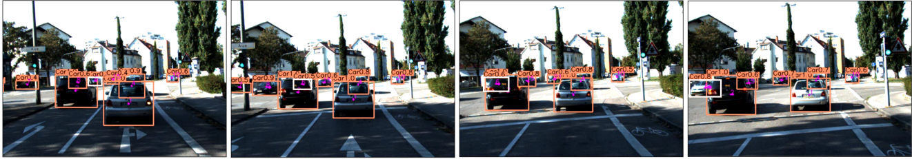
Figure 6. Qualitative results on a test sequence from the KITTI benchmark. Our approach is able to successfully track a fully occluded car on the left (id 6, highlighted in white). Please see supplementary video for a more comprehensive analysis on both datasets.
