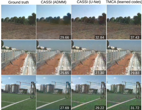
Figure 5. Examples of compressive spectral imaging reconstructions in simulation. The PSNR (dB) between the reconstructions and the ground truth images is shown in the lower-right corner.
