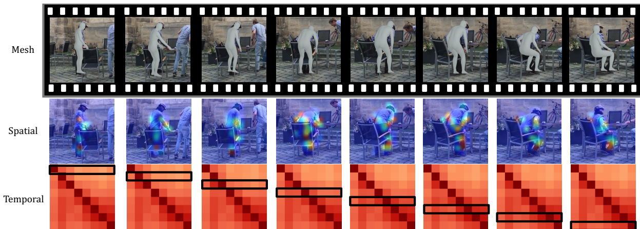
(b) Back view under cluttered background and occlusion. The heatmap of temporal attention shows relatively higher variance, indicating the current frame needs to refer to more temporal information to make up for the information lack incurred by occlusion.
