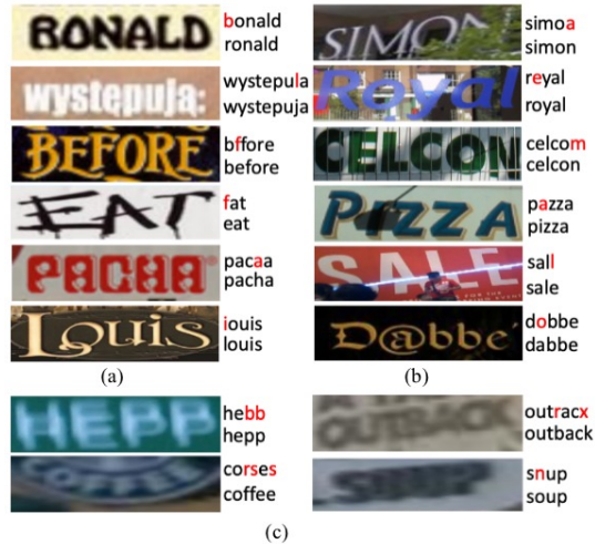
Figure 8. Recognition results with/without the use of linguistic information. The top string is the prediction of VisionLAN without MLM. The bottom string is the prediction of VisionLAN. (a): characters with confused visual cues. (b): characters disturbed by background. (c): blurred characters.
