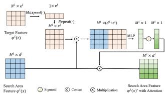
Figure 3. Illustration of Target-Guided Attention (TGA) module in MLVSNet. Our method employs an attention mechanism to embed target information into the search area in a lightweight manner.
