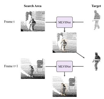
Figure 1. Illustration on how MLVSNet tracks a target on 3D point clouds. MLVSNet tracks the target object in the search area at each frame over a sequence of point clouds.
