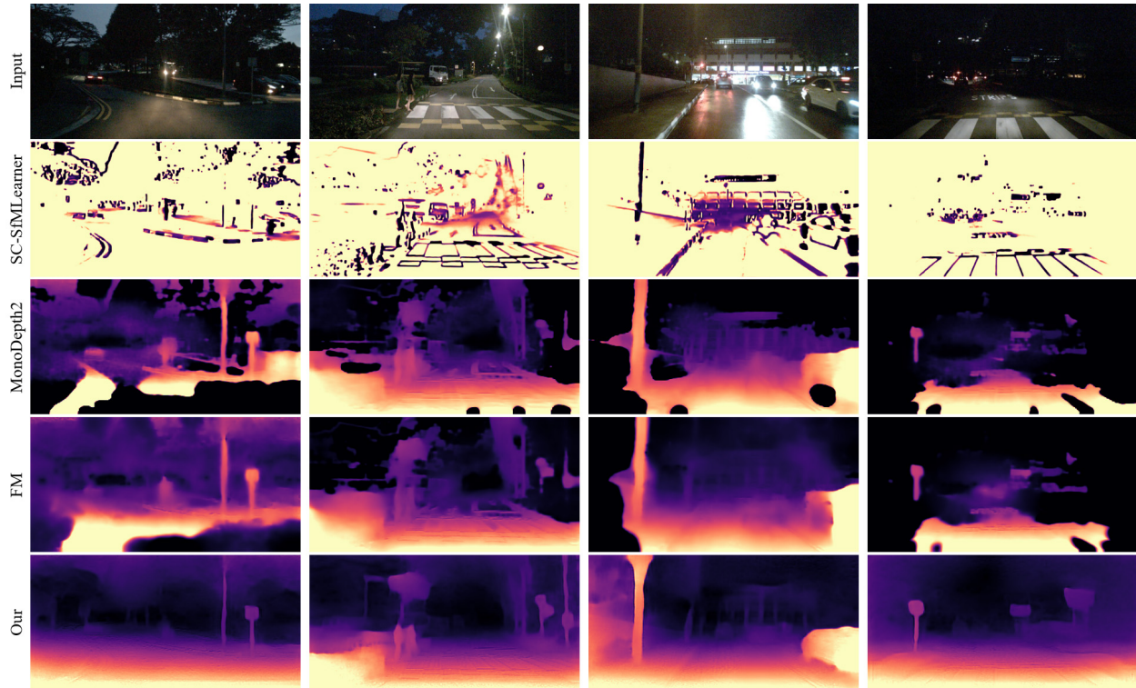
Figure 7. Qualitative results on nuScenes-Night. This dataset is more challenging due to lower visibility and more complex traffic, while our method is still able to make plausible predictions.
