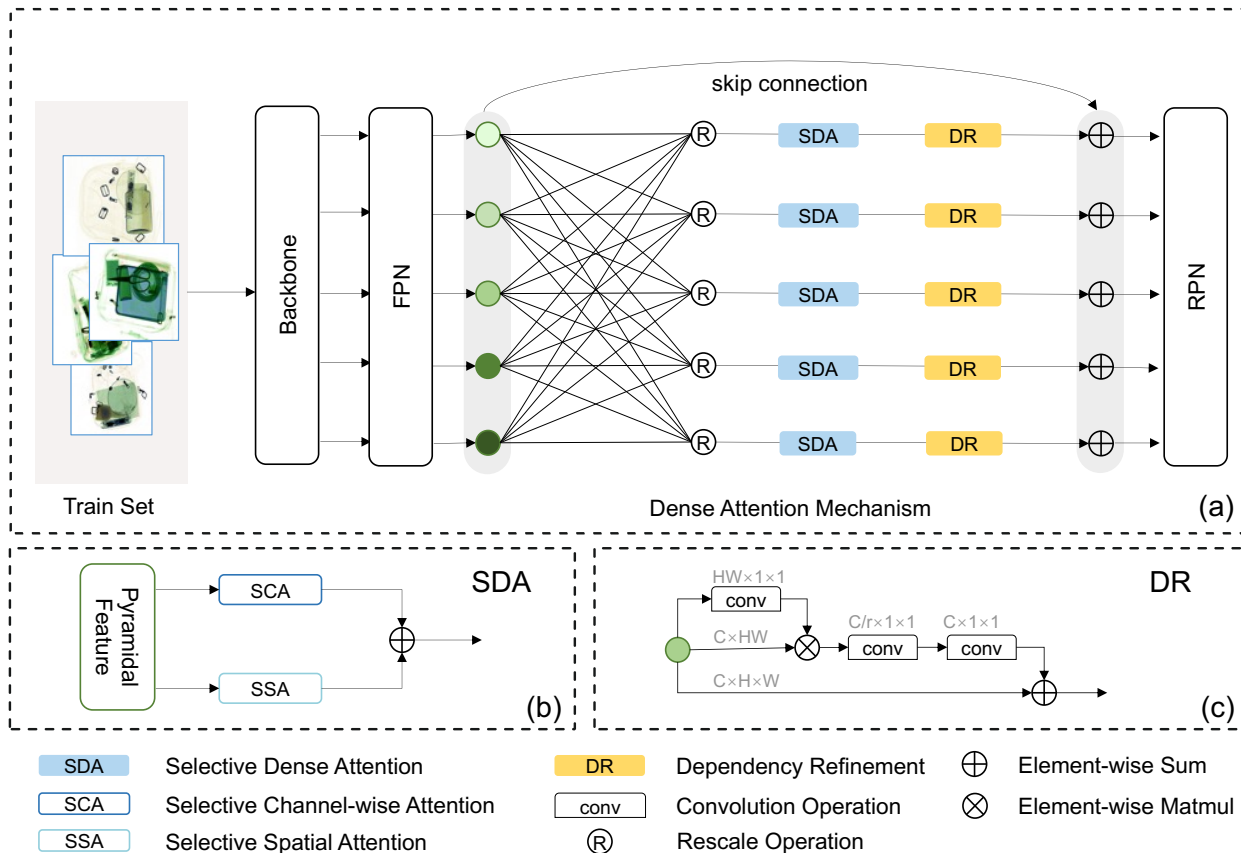
Figure 5. Network architecture. (a) The overall architecture of the proposed selective dense attention network. (b) The selective dense attention module. (c) The dependency refinement module.
