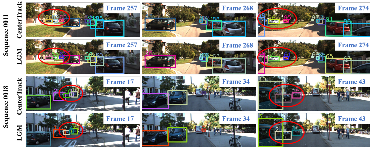
Figure 5. Examples of occlusion handling. Each row shows three frames from the same sequence. Each tracked vehicle is represented in a unique color. The number on the bounding box is the tracking ID.
