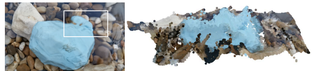
Figure 7: A failure case for the fountain scene as shown in Fig. 4. The water waves were driven by rather strong winds, and they exhibit a vortex structure (highlighted in a white box). Our method fails to produce a quality representation as a precise correspondence matching cannot be satisfied.
