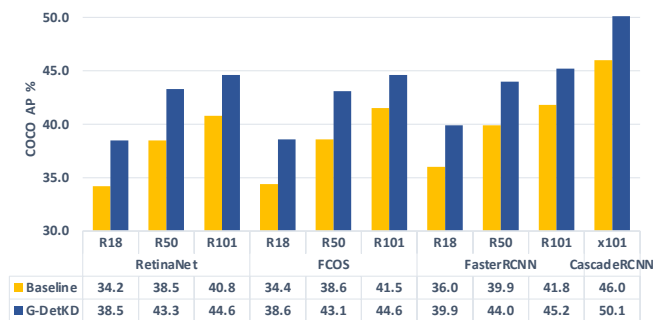
Figure 1. Our G-DetKD consistently improves the performance of detectors belonging to various categories by around 4% in AP.
