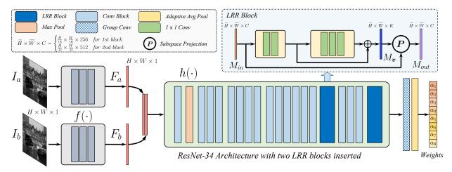
Figure 2. Our network pipeline takes grayscale image patches  $I_a$  and  $I_b$  as input, and produces 8 weights to combine 8 pre-defined homography bases to produce a homography flow as output. The network consists of two modules, a warp-equivariant feature extractor  $f(\cdot)$  and a homography estimator  $h(\cdot)$ , with 2 inserted LRR blocks to reduce the rank of the motion features.
