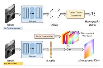
Figure 1. (a) Previous deep homography methods estimate 4 motion offsets and solve a DLT for the result. (b) We construct 8 flow motion bases by modifying matrix elements of a homography, and then regress 8 weights to combine the flow bases for the result.
