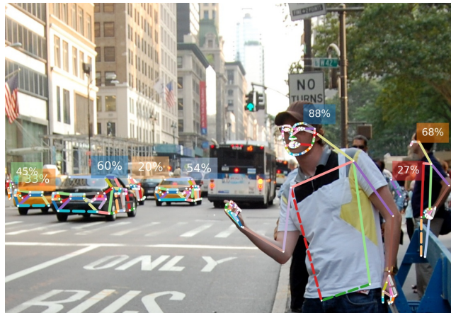
Figure 1: Our proposed keypoint weighting method for complex poses yields state-of-the-art results for whole body human pose estimation and for complex car poses, whilst running at high frame rates.
