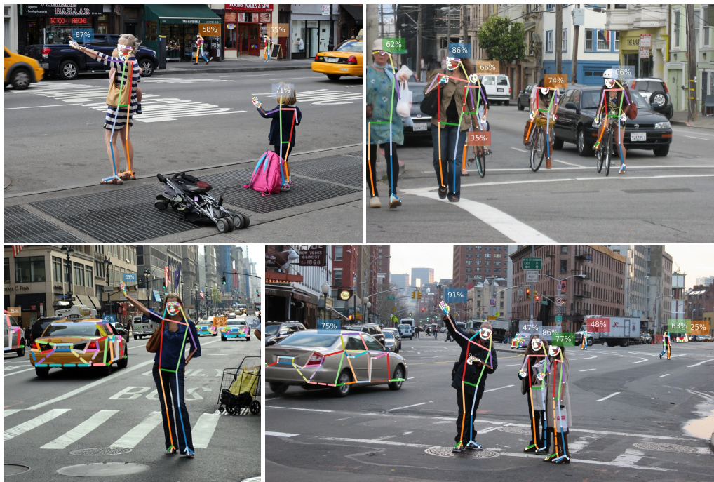
Figure 6: Qualitative results with images from the transport domain that we obtained from flickr. The two images in the bottom row were processed with our human and car pose estimation network.
