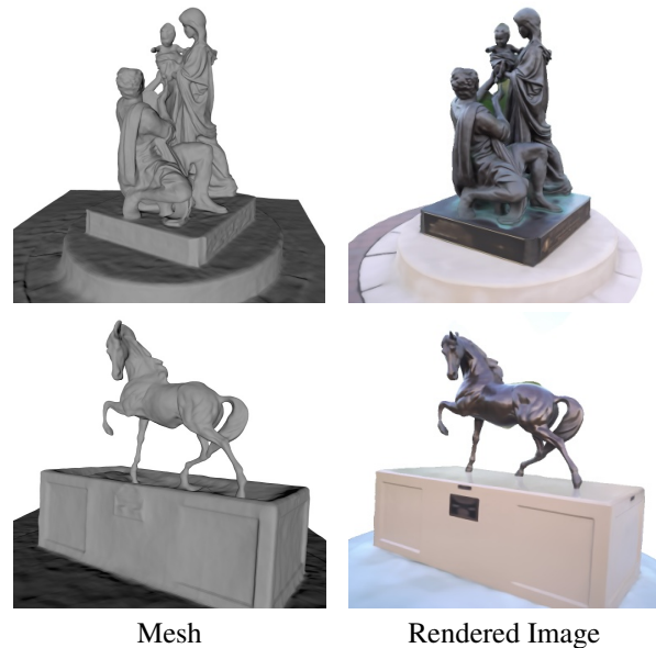
Figure 1. Our reconstructions on Family and Horse of the Tanks and Temples dataset. The proposed MVSDf is able to reconstruct correct mesh topologies with fine details for highly texture-less and reflective surfaces.
