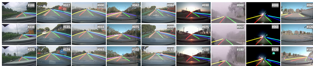
Figure 1: Our proposed Video Instance Lane Detection (VIL-100) dataset contains different real traffic scenarios, and provides the high-quality instance-level lane annotations.
