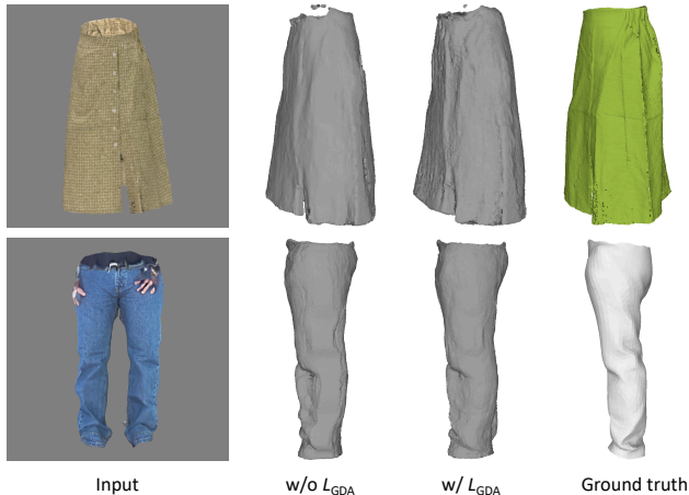
Figure 6. Visual comparison of with and without gradient direction alignment. By aligning the spatial gradient direction of the distance field, we can obtain sharper geometric details for the visible region and less artifacts for the self-occluded region.
