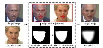
Figure 3: *Illustration of the workflow of I2G*. For each source and target image pair, a morphed mask is generated by taking a convex hull of the landmarks followed by elastic deformation and Gaussian blur. The masked region of the target image is replaced by that of the source with blending techniques [39, 35].
