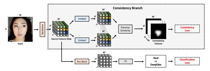
Figure 2: Visualization of PCL architecture. The consistency branch focuses on measuring the consistencies of image patches according to their source features. A classification branch is applied after the source feature map and predicts the binary score for deepfake detection.
