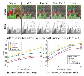
**Figure 3:** Comparison of different types and number of masks. (a) Reconstructed all-in-focus images and depth maps for cones with K=8 measurements. (b,c) Average SSIM of recovered all-in-focus images and accuracy of estimated depth for five test scenes. Quality of reconstruction improves as the number of masks increases, and learned mask patterns outperform other mask patterns.
