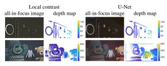
**Figure 8:** The all-in-focus images and depth maps generated by the local contrast-based method and the trained U-Net. Local contrast method uses 47.85 seconds and U-Net uses 0.0043 seconds on average.
