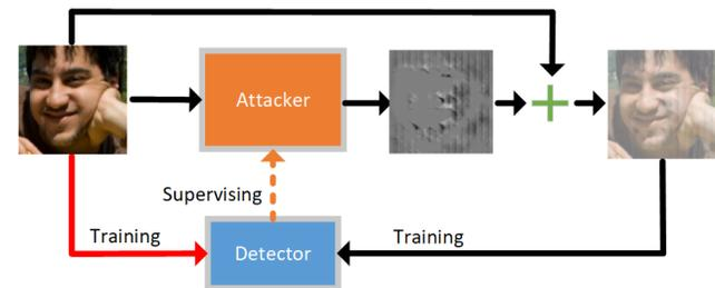
Figure 1. Insight of the proposed SAAT. The attacker generates adversarial perturbations to fool the detector, and the detector then learns to defend against attacks.
