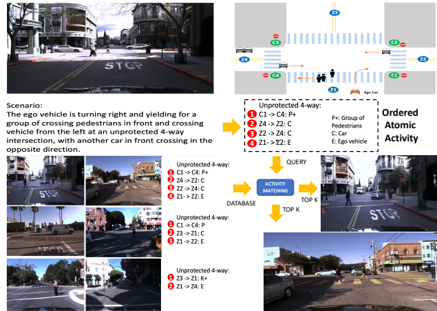
Figure 1. Ordered Atomic Activity. Instead of using natural language to describe a scenario which is verbose and time-consuming, Ordered Atomic Activity decomposes each interactive scenario into a set of ordered atomic activities, where each activity consists of an action and the corresponding actors involved and the order represents the temporal development of the scenario. The activity of "a group of pedestrians crossing in front" is represented as C1 \rightarrow C4: P+ , where C1 and C4 are the two corners, \rightarrow denotes the moving direction and the actors P+ (a group of pedestrians) perform the action. We denote the temporal development in a scenario by tagging the order of activities based on their occurrence. Ordered Atomic Activity also enables efficient scenario retrieval for applications such as scenario-based assessment.
