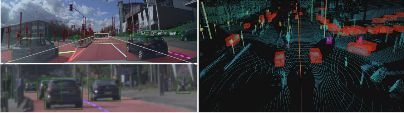
Figure 3: One *Frame* overlaid with multi-task annotations (top-left) and a zoomed-in version (bottom-left), highlighting annotated dynamic objects and lane instances at long distances. We also show the LiDAR point cloud with annotated 3D boxes and 200 m of future trajectory for the ego-vehicle (right) from the same *Frame*.
