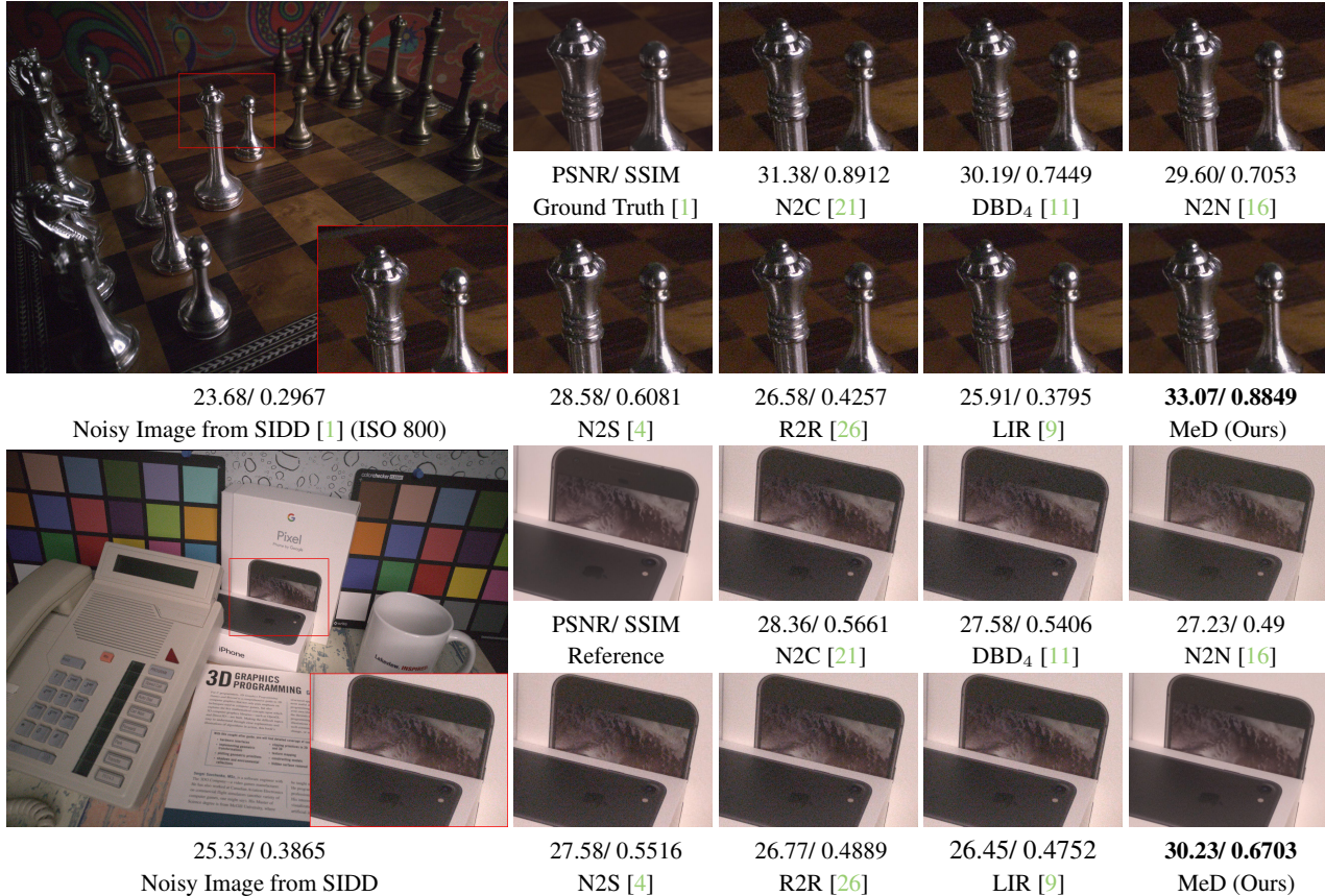
Figure 4. Real Noise Removal Example of SIDD [1] . All the methods are trained with Noise Pool on the DIV2K [2] dataset. It can be seen that the proposed MeD can remove much real noise even without training with real-noise distribution (zoom in for a better comparison).
