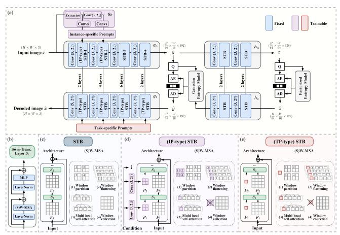
Figure 2. Overall architecture of our proposed method *TransTIC* and the detailed design of STBs.
