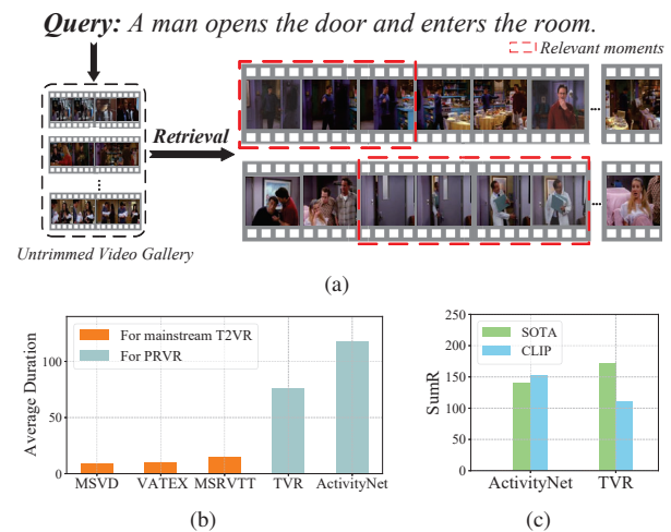
Figure 1. (a) An illustrative example of the PRVR task; (b) Mean values of video duration of different datasets; (c) Performance comparisons between the state-of-the-art (SOTA) [8] and the vanilla CLIP-based [2] methods, where CLIP shows huge performance divergences for different PRVR datasets.
