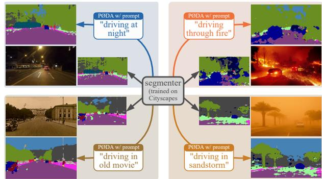
Figure 1. **Zero-shot adaptation with prompt.** PØDA enables the adaptation of a segmenter model (here, DeepLabv3+ trained on the source dataset Cityscapes) to unseen conditions with only a prompt. Source-only predictions are shown as smaller segmentation masks to the left or right of the test images.
