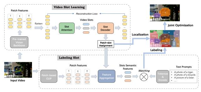
Figure 2. **Proposed framework.** Given an input video, we first localize objects by slot attention with a video encoder pretrained with self-supervision. Next, we extract semantic features for each slot by a patch-based CLIP finetuned from its vanilla version. Then, slots are named by matching slot semantic features to text features from a curated list of text prompts. Finally, the named slots are optimized to alleviate over-segmentation caused by part-whole hierarchies.
