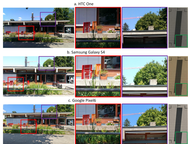
Figure 1: Sample images of the identical scene from our benchmark captured using different devices. The training and testing images are captured in hand-held mode in the wild, while the optical patterns, e.g. PSF, are obtained under controlled conditions with a fixed tripod 2 meters apart for benchmarking purposes.
