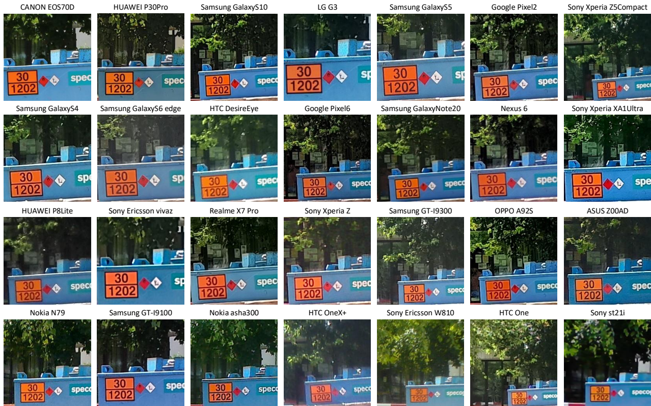
Figure 2: Smartphone Camera Sensor Quality Assessment Dataset (SQAD) . We present 224 \times 224 sized crops extracted from our dataset consisting of images captured by 29 different mobile devices. Images are arranged in descending order of resolution. Orange block scales vary due to differing image dimension settings on smartphones. Perceived sharpness relates more to PSF than resolution. The image taken with Sony Ericsson T630 is in the supplement due to its small size.
