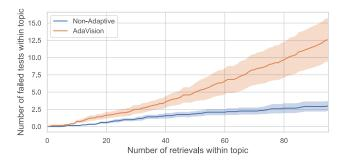
Figure 4: Average number of failures accumulated within a topic over the course of 100 retrievals, comparing ADAVI-SION with a non-adaptive baseline. ADAVISION is significantly more effective at finding failed tests, because it is able to quickly surface more failures once a few are found. Standard error is over 12 topics.
