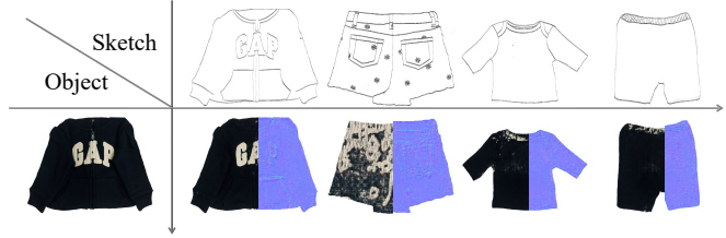
Figure 11: Failure cases. Our method struggles when the training object and testing sketch exhibit vastly different patterns. For example, given a hoodie with large letter patterns, our model reconstructs the training object (1st column) but fails to fill in the color within the flower pattern (2nd column) or to generate uniform texture around the neckline (3rd column) or the waistband (4th column).
