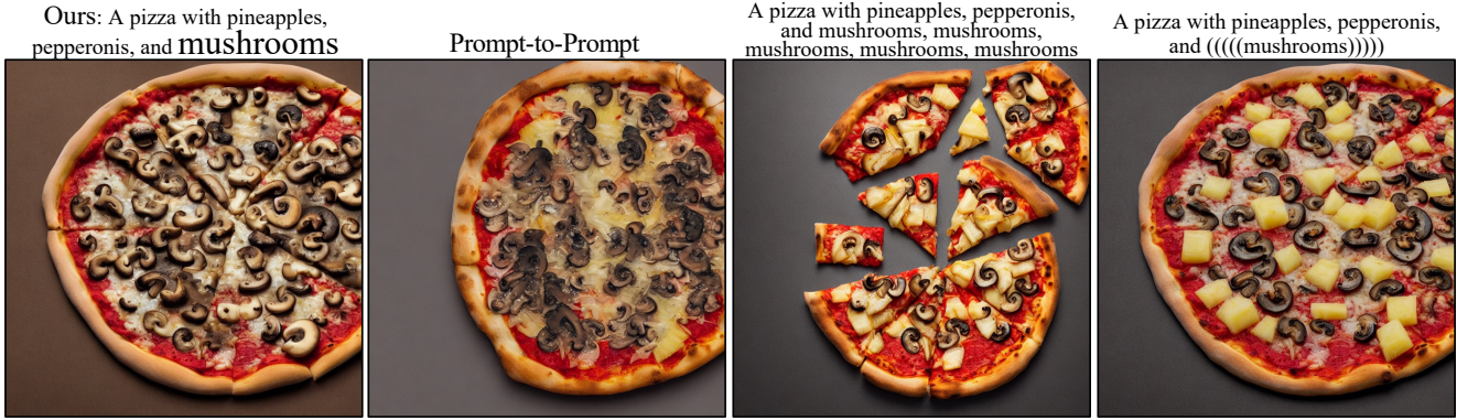
Figure 9. Qualitative comparison on token reweighting. We show images generated by our method and Prompt-to-Prompt using token weight of 13 for ‘mushrooms’. Prompt-to-Prompt suffers from artifacts due to the large weight. Heuristic methods like repeating and parenthesis do not work well.
