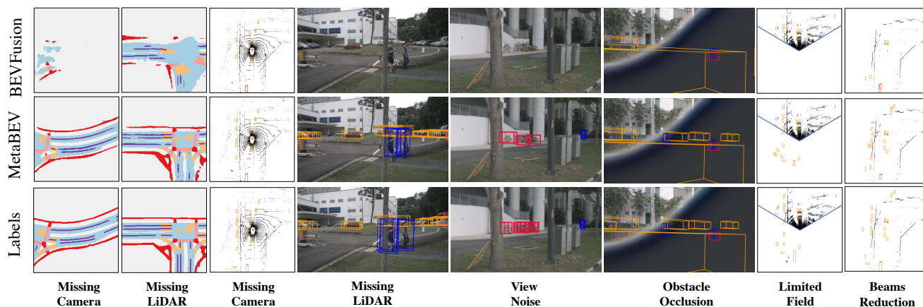
Figure 1. Selected 3D prediction results under various sensor failures. MetaBEV shows stronger robustness on both map segmentation and 3D detection compared to the representative multi-modal method, e.g., BEVFusion [25]. Notably, in case of an entire sensor absent (e.g., Camera or LiDAR), MetaBEV provides satisfactory outcomes while existing methods fail to. Top two rows: 3D prediction results. Bottom row: the corresponding ground truths.
