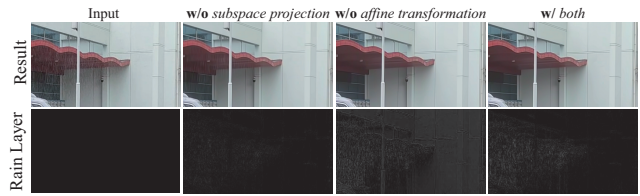
Figure 9: Ablation study of the robust low-rank tensor recovery model. The first row represents the deraining results, and the second row is corresponding rain. The first column is the original rainy frame and the remaining three columns represent the model without subspace projection, without affine transformation and full RLTR.
