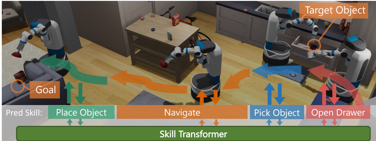
Figure 1: A Fetch robot is placed in an unseen house and must rearrange an object from a specified start to a desired goal location from egocentric visual observations. The robot infers the drawer is closed and opens the drawer to access the object. Next, it picks the object, navigates to the goal, and places the object. The Skill Transformer is a monolithic “pixels-to-actions” policy for such long-horizon mobile manipulation problems which infers the active skill and the low-level continuous control.
