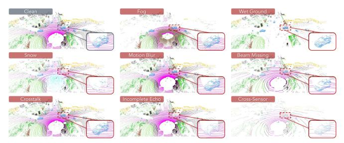
Figure 1: Taxonomy of the **Robo3D** benchmark. We simulate *eight* corruption types from *three* categories: 1) *Severe weather conditions*, such as fog, rain, and snow; 2) *External disturbances* that are caused by motion blur or result in the missing of LiDAR beams; and 3) *Internal sensor failure*, including LiDAR crosstalk, possible incomplete echo, and cross-sensor scenarios. Each corruption is further split into *three* levels (light, moderate, and heavy) based on its severity.
