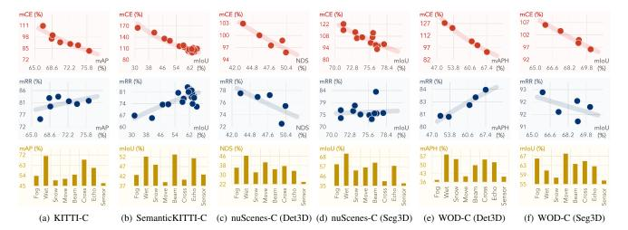
Figure 2: Benchmarking results of *34* LiDAR-based detection and segmentation models on the *six* robustness sets in Robo3D. Figures from top to bottom: the task-specific accuracy (mAP, mIoU, NDS, mAPH) *vs.* [first row] mean corruption error (mCE), [second row] mean resilience rate (mRR), and [third row] sensitivity analysis among different corruption types.
