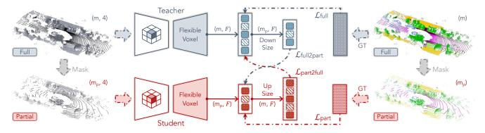
Figure 5: The proposed density-insensitive training framework. The "full" and "partial" point clouds are fed into the teacher branch and student branch, respectively, for feature learning, while the latter is generated by randomly masking the original point cloud. To encourage cross-density consistency, we calculate the *completion* and *confirmation* losses which measure the distances of sub-sampled teacher's prediction and interpolated student's prediction between the other branch's outputs.
