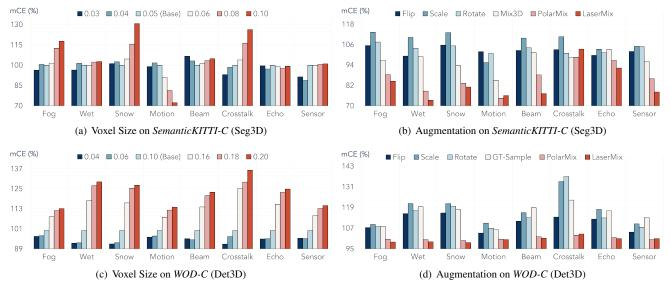
Figure 4: Corruption sensitivity analysis on *voxel size* (a & c) and *augmentation* (b & d) for the baseline LiDAR semantic segmentation and 3D object detection models [12, 82]. Different corruptions exhibit variances under certain configurations.
